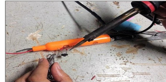
Figure 14: Soldering the stylus' electronic components
