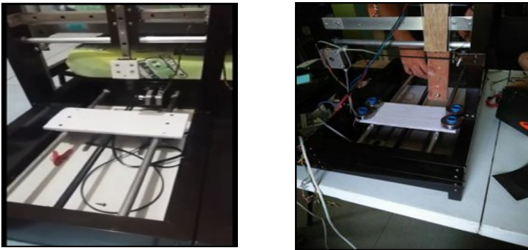
Figure 30. Fixing Motors in the Body Frame and Putting Belts and Platforms and other parts
