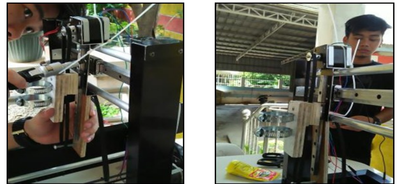
Figure 32. Fixing the Drill in the Z-axis
